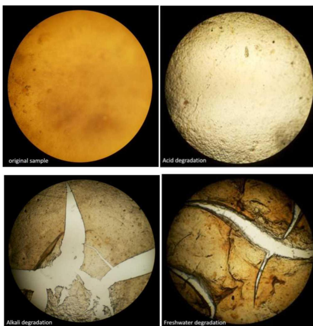
Figure 2 Microscopic images of bioplastics films; biodegradation test in different media
